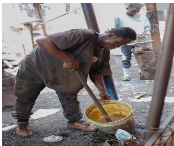
Plate 1b. Artisan quenching a metal object in a bucket of dirty water
