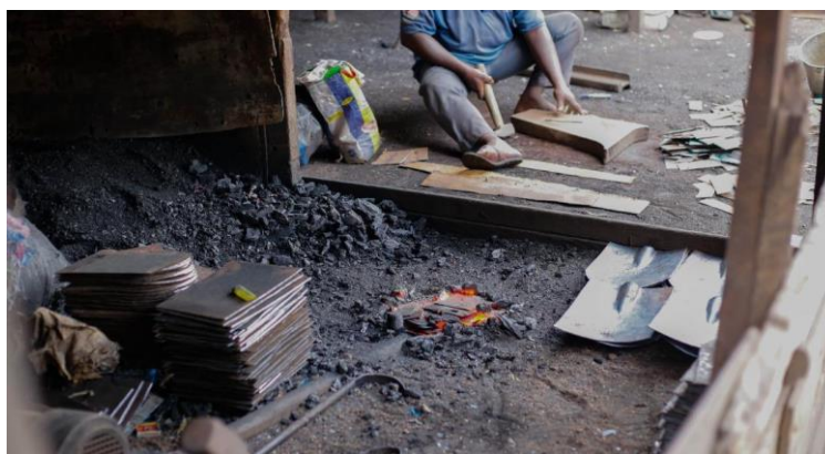
Plate 1a. Furnace made in the ground.
