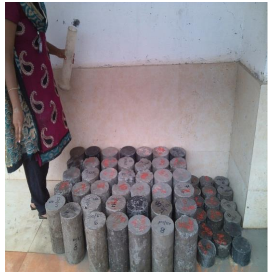
Fig 7.1 Cylinders after Curing Left For Air Drying For 24 hrs.
