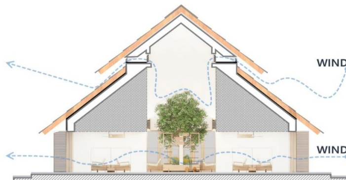
Figure 7 shows the design of openings for natural ventilation through the interior of the building.
