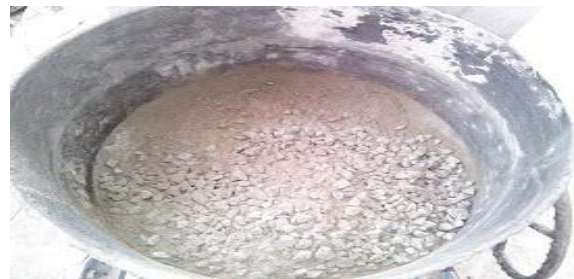
Figure 3.1 Mixing of coarse aggregate and fine aggregate
