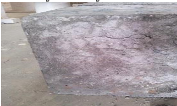
Figure 4.3 Cube after failure under Compression load.
