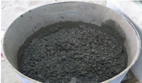
Figure 3.4 Mixing of Solution to aggregates and glass fibres
