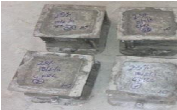
Figure 4.1 Casting of Cubes
