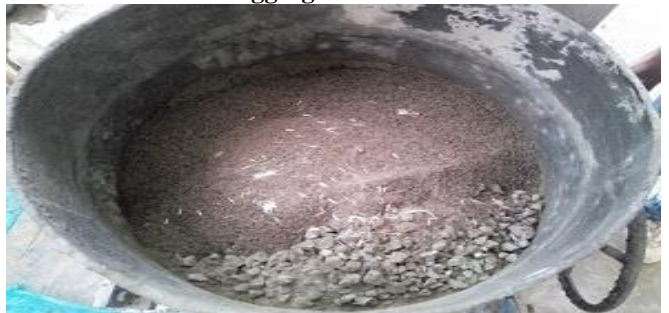
Figure 3.2 Mixing of glass fibres, Cement, coarse & fine aggregate
