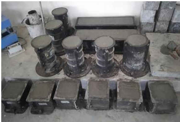
Figure 3.5 Casting of M30 grade Glass Fibre Reinforced Concrete
