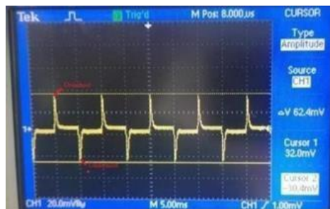
Fig 8; Load Transient of O/P-2(5V/2A) at 36V Input
