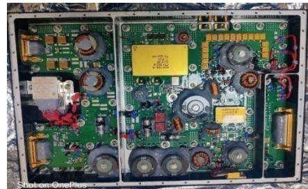
b) Top view of the forward converter when the load is at 100%
