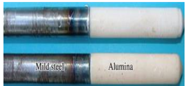
Figure 3.2: Alumina and steel weld joints
