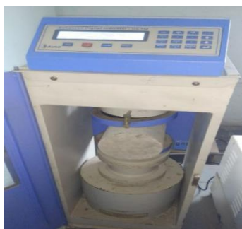
Fig 4.7 Split tensile strength test
