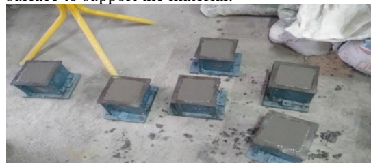
Fig 4.5 casting the cubes
