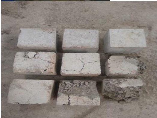
Fig 4.6 compressive testing machine and cubes after test
