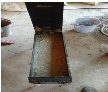
Fig 4.3 L - box U box test
