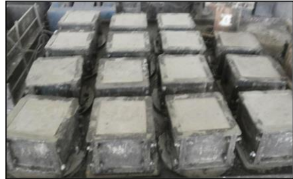
Figure 4.2 Casting of concrete cubes for CS
