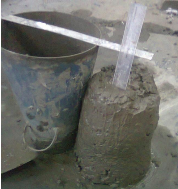
Figure 4.3 Slump of fresh concrete
