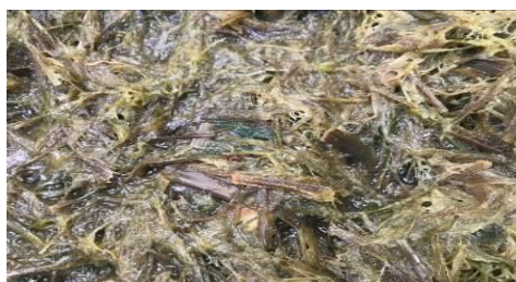
Fibrous pulp boiled in sodium hydroxide
