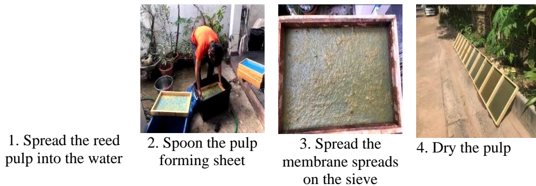
Figure 6 The process of spooning the pulp to make sheets of material
