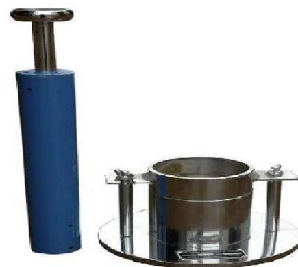
Fig 3.1. Modified Proctor test apparatus
