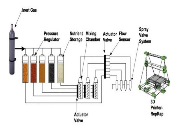
Fig(i):3.d printing mechanism
