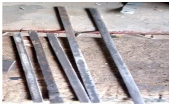
Figure 31: Scrap Strip Metal Used For The Saw Frame
