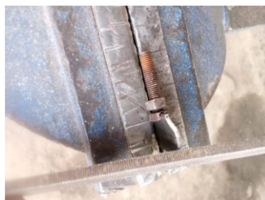
Figure 58: Filing of edges of welded thumb screw with hand file and bench vice
