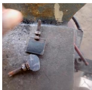
Figure 57: Welded thumb screw
