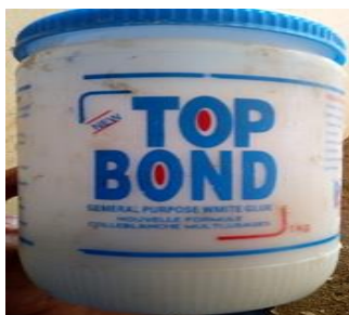
Figure 36: PVA White Glue Was Used With Saw Dust To Hold Firm The Handle Of The Saw Frame
