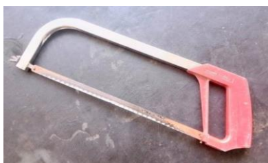
Figure 21: Hacksaw With Blade Used For Cutting
