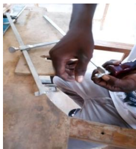
Figure 76: Fixing Blade Into The Finished Saw Frame
