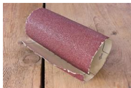
Figure 28: Sand paper was used in smoothing the surface of the metal and wood
