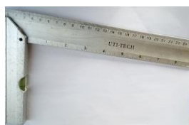
Figure 27: 90° angle ruler was used in checking straightness of the work through the angles
