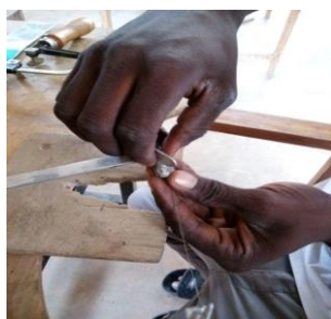
Figure 77: Checking For Tension In The Fixed Blade (C,D)
