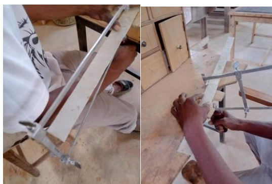
Figure 78: Piercing with the new jeweller's saw frame (A, B) Source: Researcher's studio 2022.
