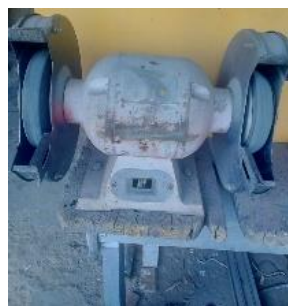
Figure 42: Grinding Machine For Smoothen Surface And Edges Of Metal Used For Frame Source: Researcher's Studio 2022.
