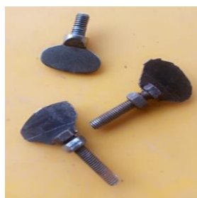
Figure 59: Finished thumb screw Source: Researcher's Studio 2022.
