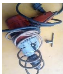
Figure 23: Electrical Hand Drill Machine Used For Creating Hole
