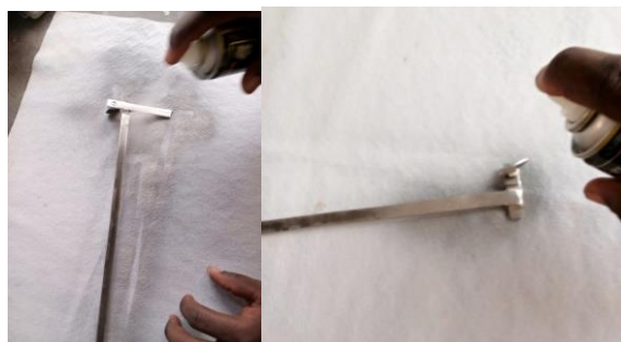
Figure 71: Spraying The Components Of Saw Frame With Silver Spray
