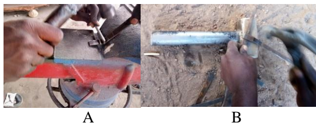
Figure 47: using of hammer to align metal (AB)
