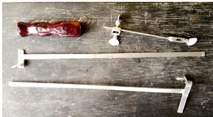
Figure 79: Dismantled jeweller's saw frame Source: Researcher's studio 2022.
