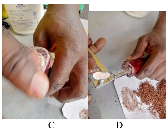
Figure 74: Applying Glue And Saw Dust Into The Slot In The Wooden Handle And Putting In The Saw Frame To Complete The Process.
