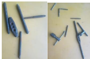
Figure 26: Screw Thread Tap Wrench For Creating Thread Slot
