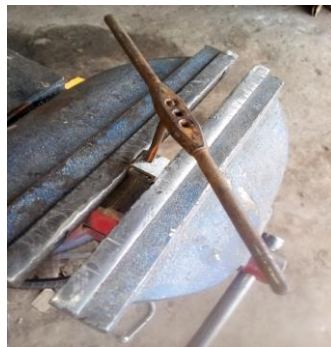
Figure 54: Using thread tool to create thread space to accommodate thumb screw on the frame (C)
