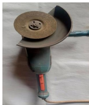
Figure 39: Cutting Machine Was Used For Slitting And Cutting Metal
