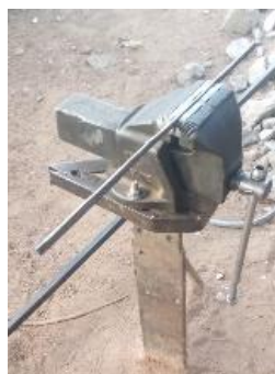
Figure 40: Bench Vice Was Used For Hold Firm Metal
