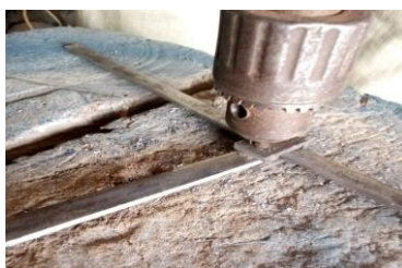
Figure 49: Creation of hole with the use drilling machine
