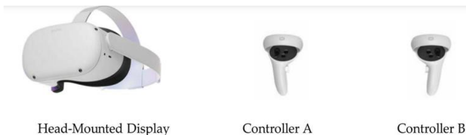
Figure 1. Oculus Quest 2. From the left, the head-mounted display, the left controller (Controller A), and the right controller (Controller B)
