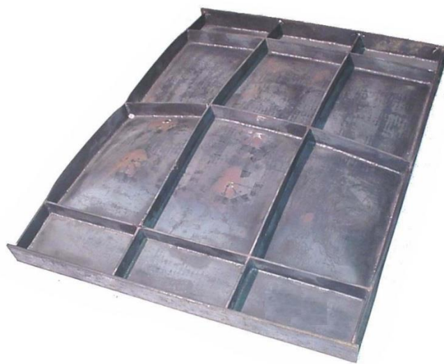
Fig.9 Experiment's failure shape (Shanmugam et al., 2014).
