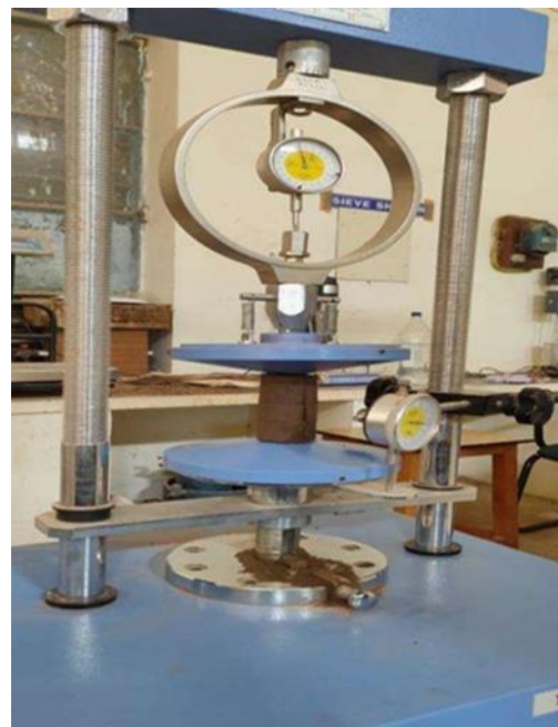
Figure 2: Unconfined Compressive Strength testing machine.
