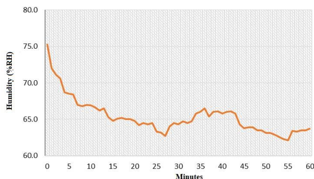
Figure 10. Humidity response graph on on-off control system
