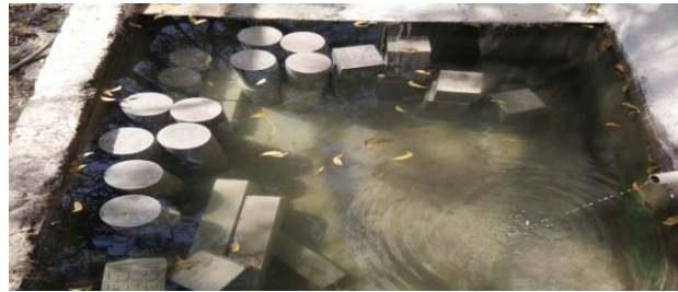
Figure 3.3 Test specimens kept for curing
