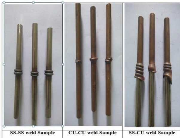
Fig 3.3 Friction welded dissimilar welded specimens
