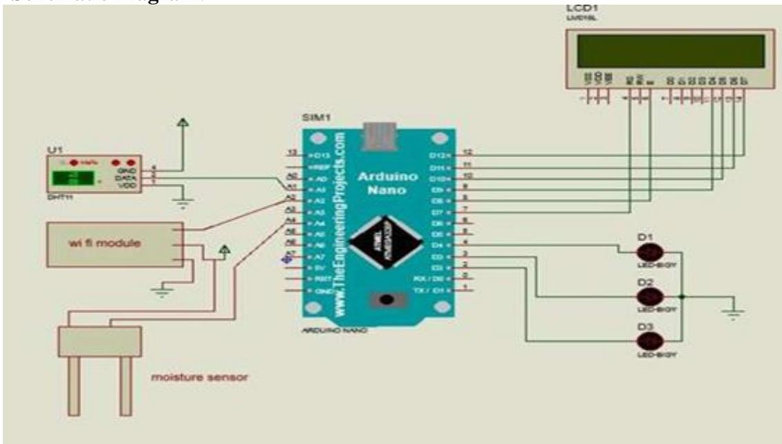
Hardware designed for greenhouse monitoring and control is used to regulate the greenhouse's environmental conditions and bring it into good shape. The greenhouse's temperature and
