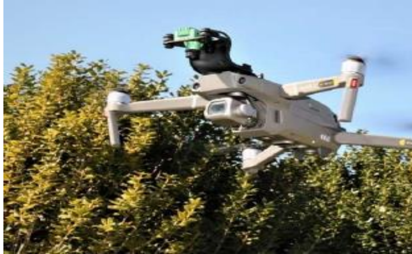
(DJI Mavic air UAV with single NDVI camera over the automatic detection)
