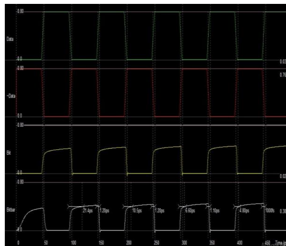
Fig 8: Simulation Result of 6T-SRAM Cell
