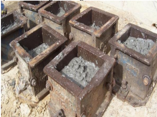
Figure 3.3. Casting of cubes
