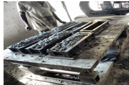
Fig3.2.: casting of specimens
