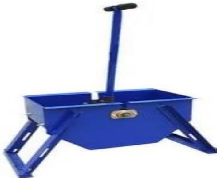
Figure 2. Represents the Manual Groundnut Shelling Machine for Small Scale Farmers [Source: shellermachine.com]
