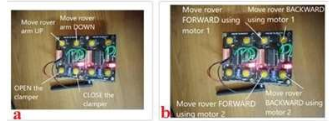
Fig.4. RF controller (remote) modes of operation for (a) End-Effector, (b) Wheel DC Motors.
