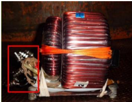
FIGURE 14(a). Coil without secondary plate in oven
