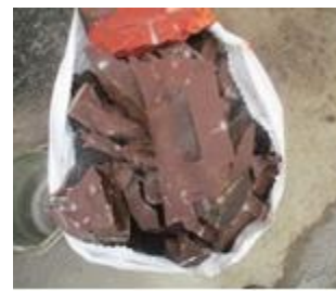
FIGURE 4(e). Broken casting
