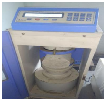
Fig 4.7 Split tensile strength test
