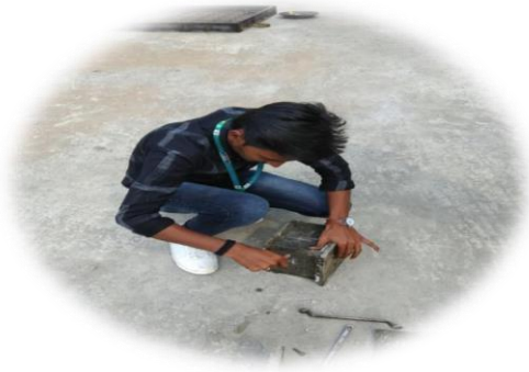
Fig: 3.8. De-moulding of specimens
