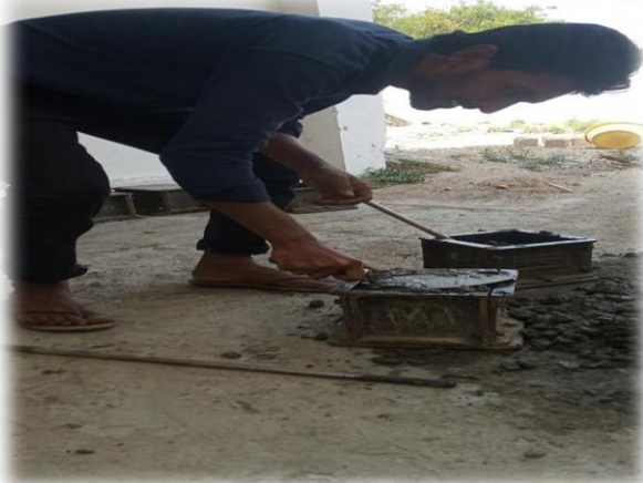
Fig: 3.5. Casting and Compaction of Cubes
