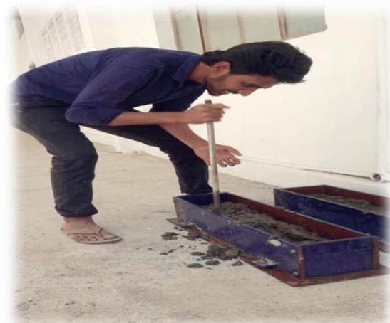
Fig: 3.7. Casting and Compaction of Beams
