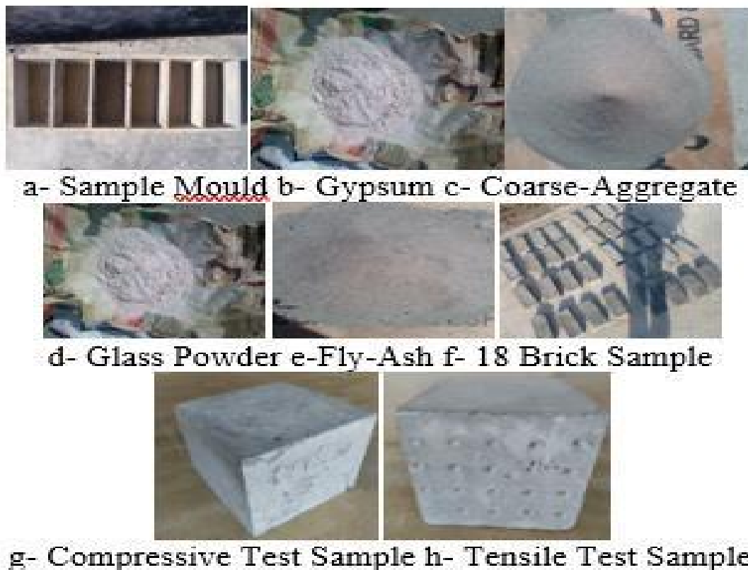
Figure 2. Detail view of Diverse Material used in Fly-Ash Building-Bricks with Samples and Mould.
