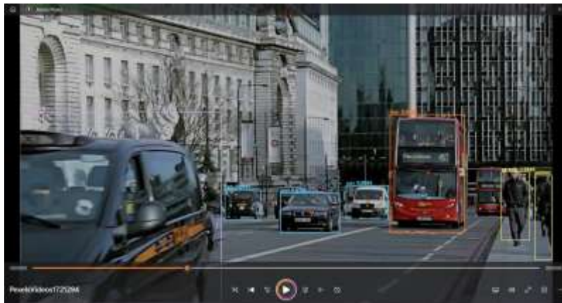
Figure 7: video frame with classification of persons, cars & buses with an accuracy of 94% ,96% & 99%
