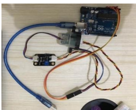
Figure 8 Turbidity Sensor Calibration Circuit
