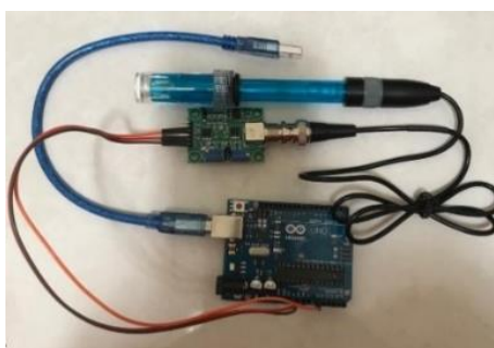
Figure 7 pH sensor Calibration Circuit
