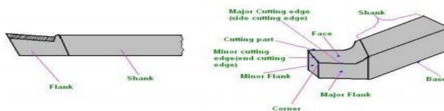
Nomenclature of a single point cutting tool
