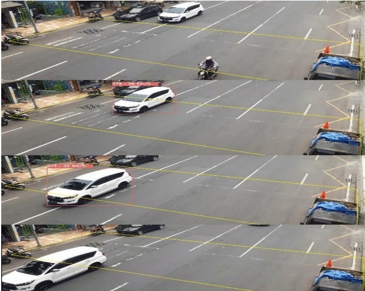
Fig. 6: The bounding boxes is only drawn per frame when the centroid of the car is inside the ground truth area marked with yellow box.
