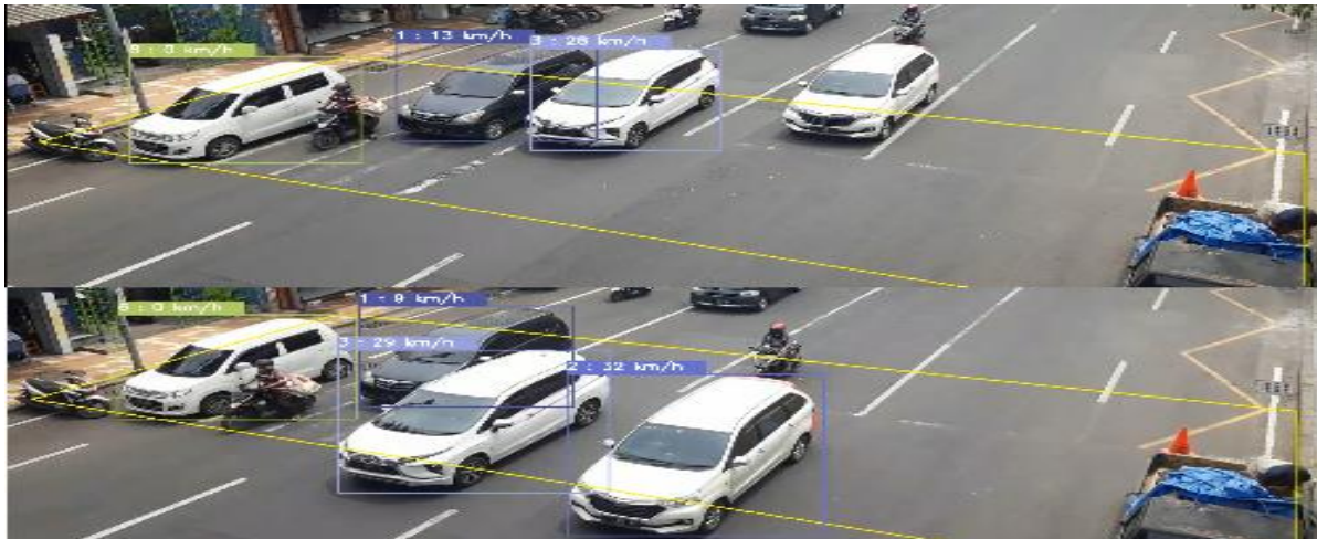
Fig. 5: A car is detected using YOLOv4, and when entering the ground truth area and if the centroid of the car is inside the area, the start bounding box is drawn as seen on the top image. DeepSORT tracks the movement of the detected car as seen on the bottom image.
