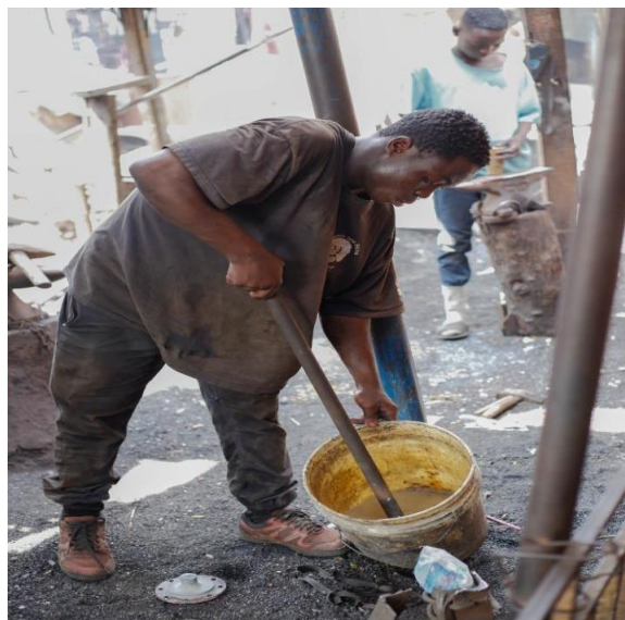
Plate 1b. Artisan quenching a metal object in a bucket of dirty water
