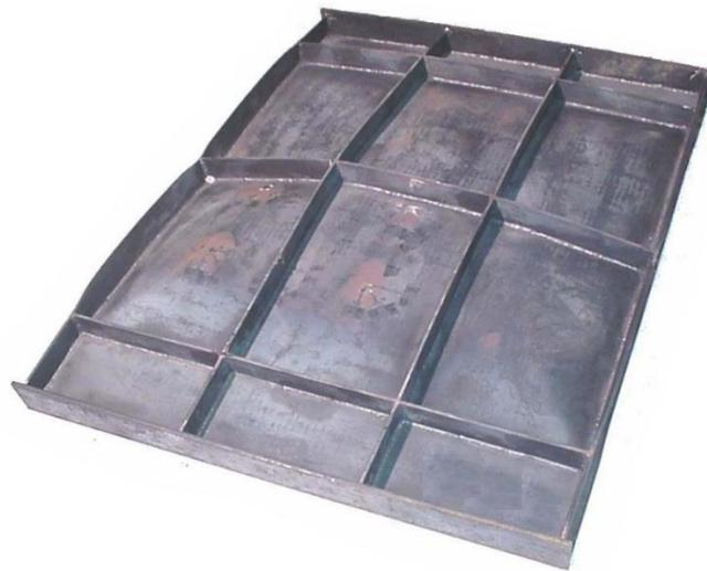
**Fig.9** Experiment's failure shape (Shanmugam et al., 2014).
