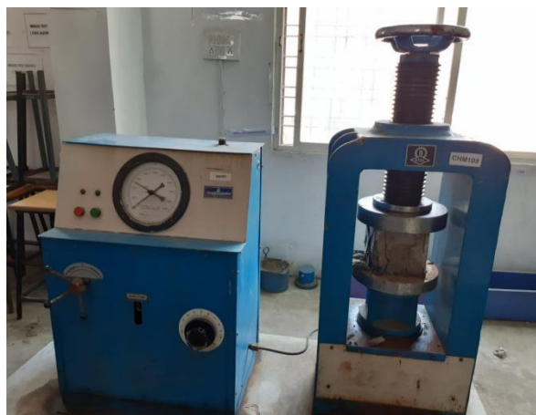
Fig. 6: Compressive strength test of cube sample.
