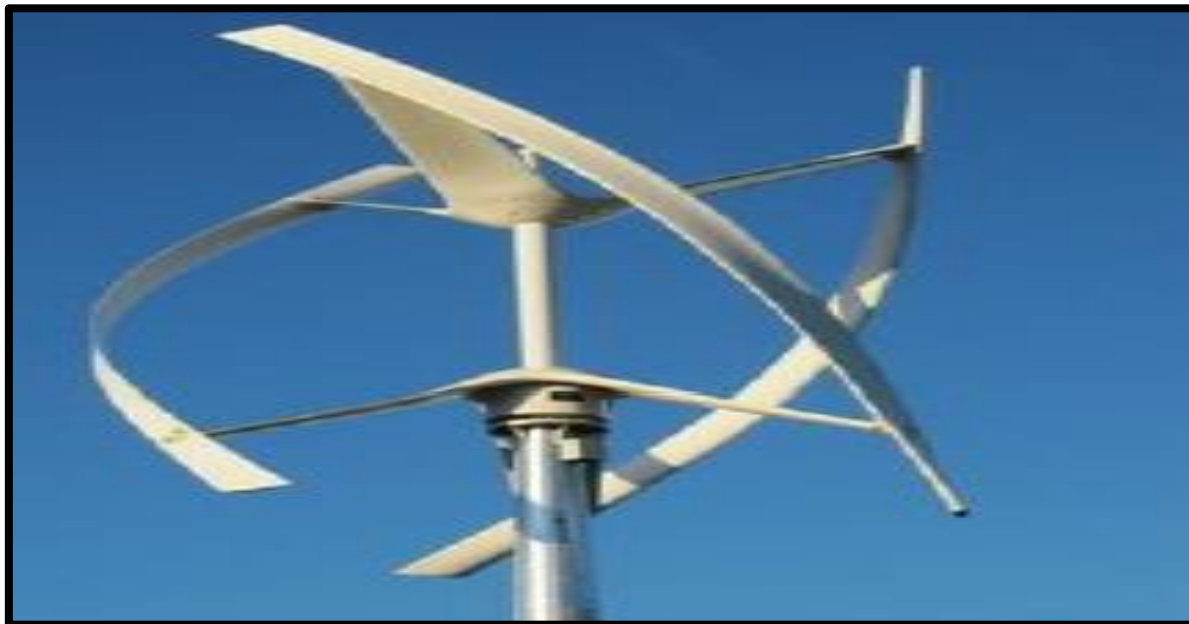
Fig 4. Vertical Axis Wind Turbine.
