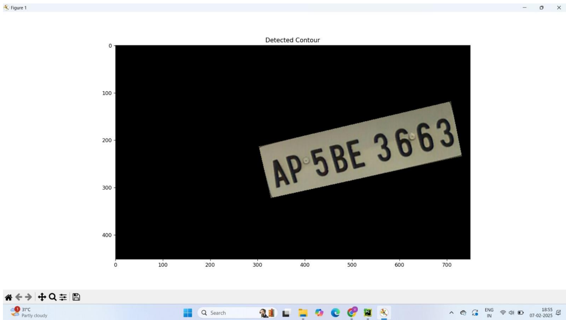
Figure 4: Find contours and apply the mark to separate the actual number plate.
