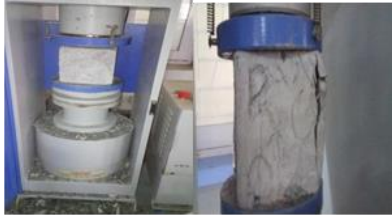
Figure 5: Testing cubes in compressive testing machine
