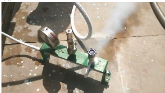
Fig. 4.4 Pressure Gauge – Globe valve setup
