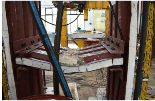
Figure 19: Crack formation in SFCC floor and wall panel
