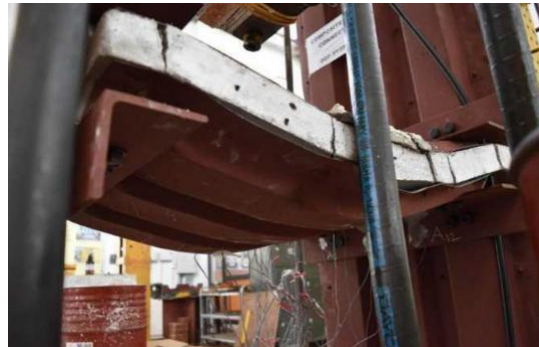
Figure 20: Deformed view of SFCC floor panel
