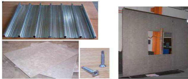
Figure 2: PSSDB wall panel (Source: Hamzah & Badaruzzaman 2009)
