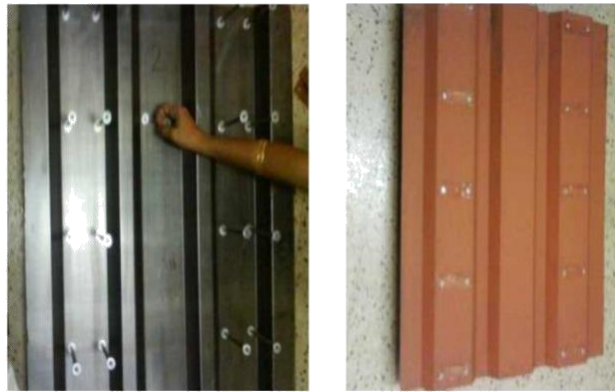
Figure 12:Assembling of SFCCP-ACL specimens
