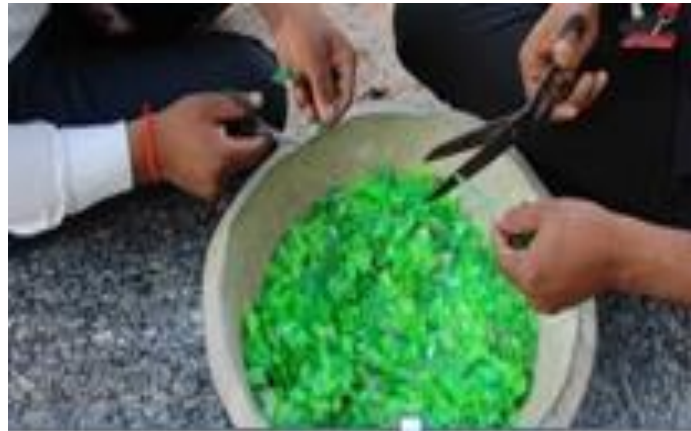
Figure 3.1 depicts the process of crushing bottles of plastic.
