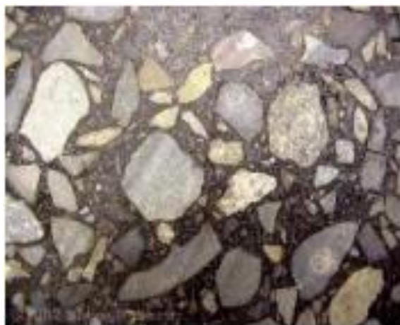
Figure:1.2.Open graded HMA
