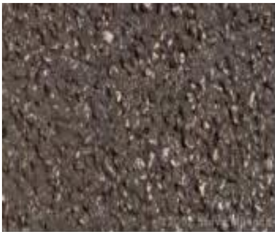
Figure:1.2.Open graded HMA
