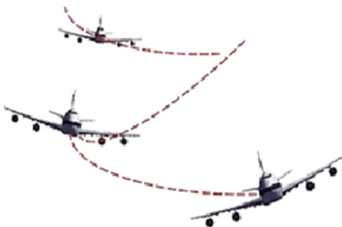
Fig2. Dutch Roll Oscillations in fixed wing aircraft
