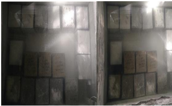
Fig. 5: Water curing of samples.
