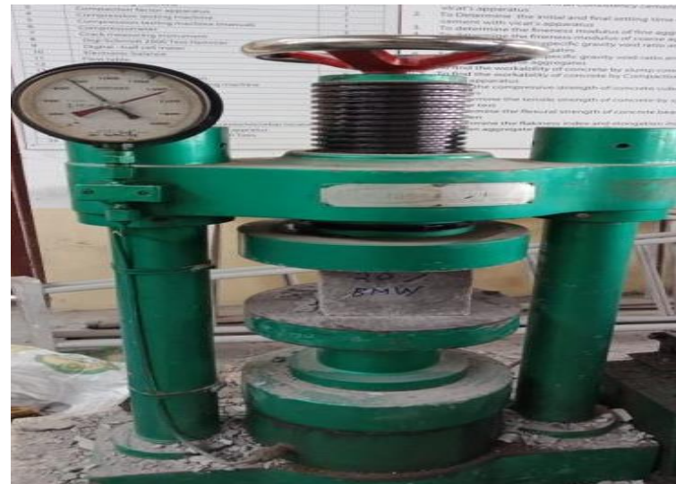
Fig. 6: Compressive strength testing of cube sample.
