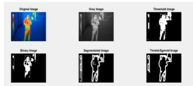
Fig. 7: Output of segmentation and threshold segmentation of a thermal camera image: From Left upper row: Original image, Gray scale image, threshold gray scale : from Left Lower row :binary image, segmented image, Threshold segmented image The additional threshold segmentation gives a better result to work further. After the image is segmented, the process of morphological opening removes small artifacts. Next process on the binary image is to select the interconnected group of pixels which maybe the object we are trying to detect and then it is labeled and it's all properties like length, width height are measured so that we can assume what actually the image is, This process known as connected component labeling (CCL).
