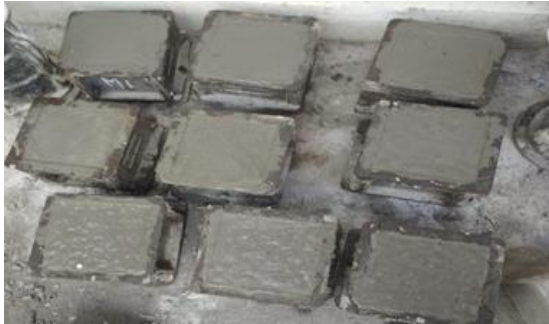
Figure-3.4 Casting of cubes
