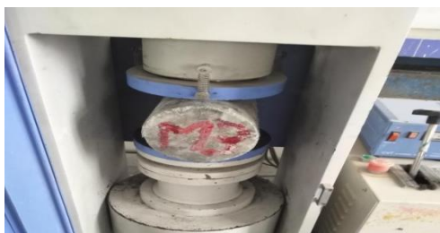
Figure-3.7 Split tensile test
