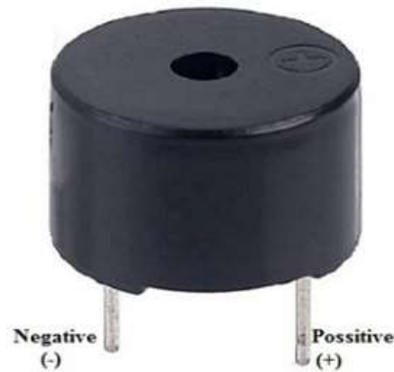
Fig 10. Buzzer Pin Configuration
