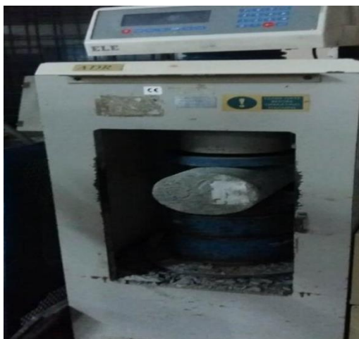
Fig. 2.10. Split tensile strength Test
