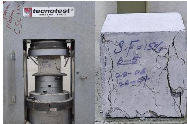
Figure 6: Cubes specimen under testing
