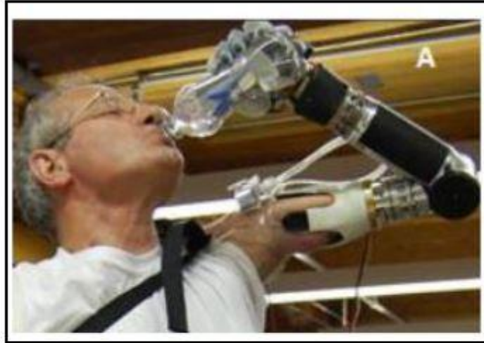
Figure 3: Myoelectric upper limb device.
